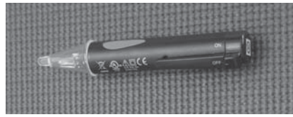
Figure 21 - Use a non-contact circuit tester to check for electrical power.
